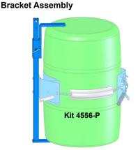
Install Bracket Assembly Kit 4556-P to prevent drum from slipping length-ways. Required to safely handle a RIMLESS 55-gallon (210 liter) plastic drum. Also recommended to more securely hold fiber drum. Adjusts for 31" to 39" (78.7 to 99 cm) tall drum.
