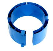
This **Diameter Adapter** allows you to handle a 19" (48.3 cm) diameter drum with model 185G-HD. Simply place Diameter Adapter into the drum holder. When dispensing is complete, simply lift Diameter Adapter out of drum holder to return to handling a 55-gallon (210 liter) drum.
