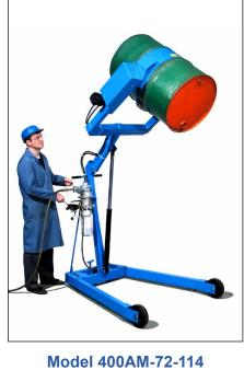
Hydra-Lift Karrier with spark resistant parts, with 72" (183 cm) lift height, air powered drum lift and tilt control.
