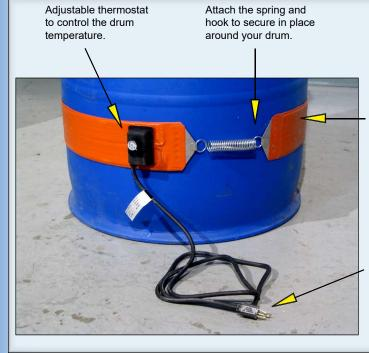
Tough fiberglass reinforced silicone rubber band is flexible, chemical resistant, and easy to keep clean. Heater band conforms to the drum surface, held in contact by spring tension. Heaters have a 4" (10.16 cm) wide with heating elements
