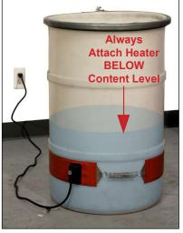
Drum heaters MUST be properly positioned BELOW the content level in the drum. Drum heater provides uniform heat over the 4" (10.16 cm) wide band around drum.
