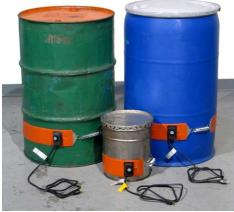
To attach to your drum, simply wrap drum heater around below level of contents within drum, and engage the spring and hook to hold it in place. transfer through drum sidewall to material inside. They are more flexible than metal band heaters, and therefore able to conform to the drum's
