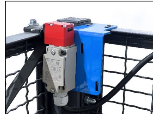
p Close enclosure and verify that the key aligns properly with the switch. If key is not aligned properly, adjust accordingly. Key may be adjusted by loosening its screws and moving, then re-tightening screws. Use zip ties to retain cable from switch to control station.
