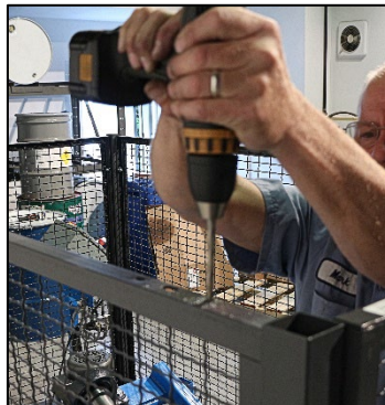
Drill holes for switch mounting plate.
