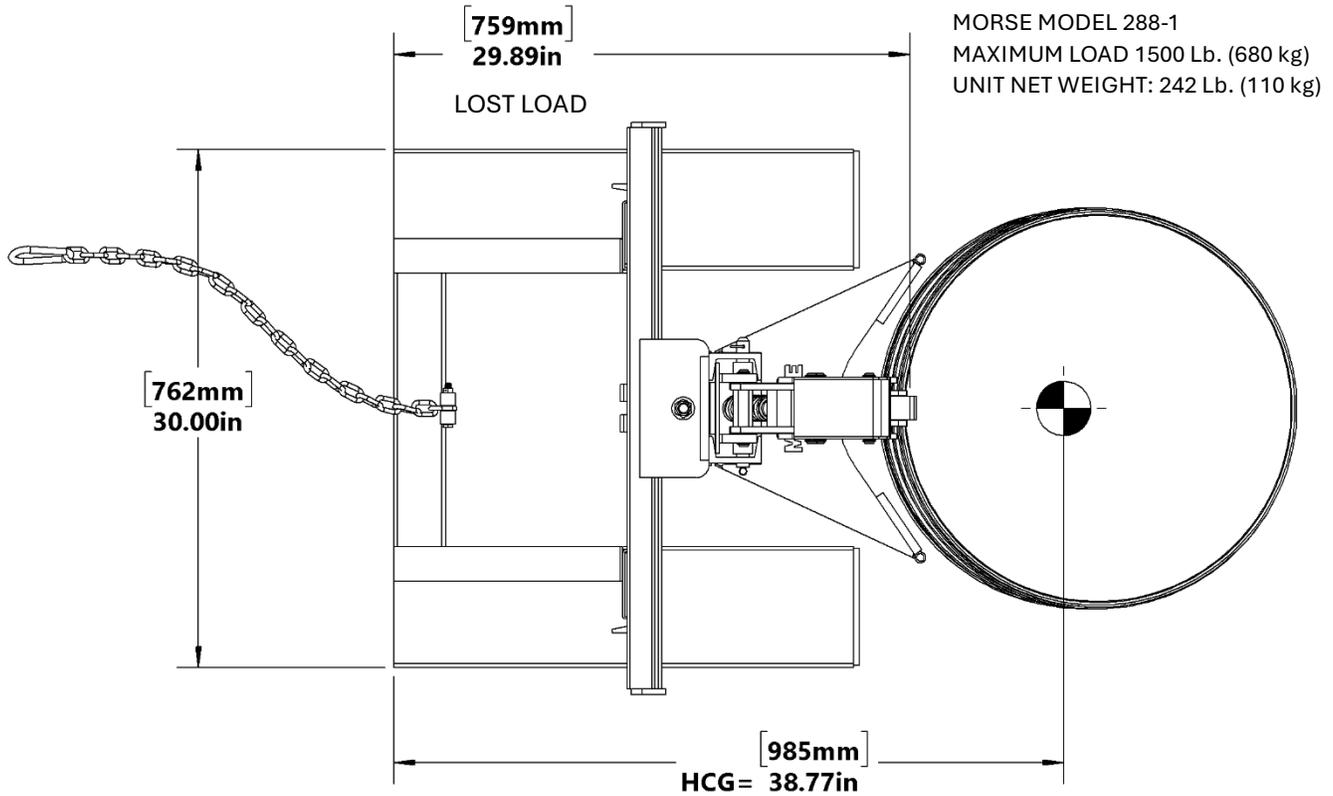
IN THIS CONFIGURATION, THE LOAD CENTER OF THE DRUM IS APPROXIMATELY THE SAME AS HCG
