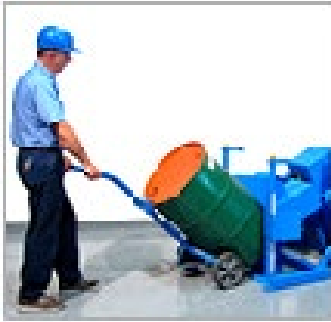
Figure 5.1 Load drum with drum truck
