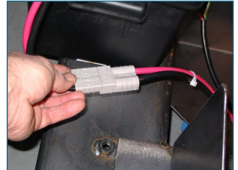
13. Plug battery to pump. Test unit function for forward and reverse.
