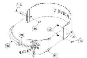
MORCINCH<sup>™</sup> Drum Holder (5000-P) has Cinch Chain and Ratchet to secure around drum.
