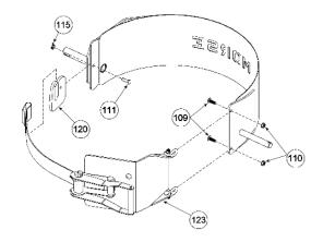
Install Kit 5115-P to convert to Web Strap and Ratchet to secure around drum.
