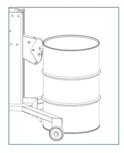
3. With drum held off the floor, push drum lifter to deliver drum. Avoid unreasonably rough or non-level surfaces. Move at moderate speed. Carry drum only high enough to avoid contact with the floor or obstacles. Push (rather than pull) loaded unit when possible for transporting. Pulling unit should be limited to maneuvering at short distance.
