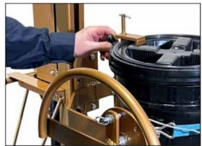
5. Crank the cable winch to lift pail about 6" (15 cm) off the floor.
