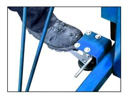
Secure pail in holder: Drape web strap around pail and engage web strap hook in eye. Use ratchet to tighten web strap around pail.
