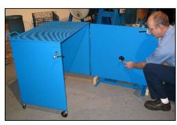
Step 7: Align each self drilling screw near the center of the angle frame.
