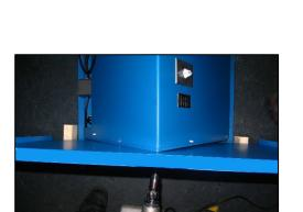
Step 8: Screw 5 self drilling screws through back panel and into the angle frame.
