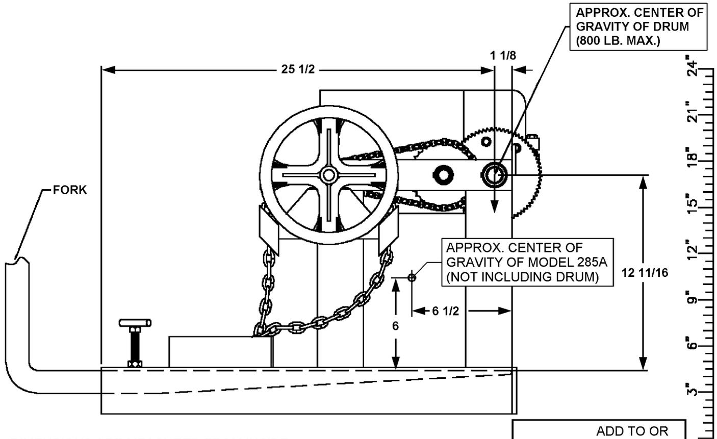
DIMENSIONS ARE MEASURED FROM INSIDE OF FORK TUBE END. THIS WILL GIVE A FIXED POINT TO WHICH LOST LOAD DATA CAN BE DETERMINED. (FORKS MUST BE TOUCHING THIS FORK TUBE END.)
