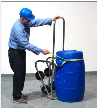
Secure optional strap (shown on model 160-SS) around a rimless drum.
