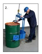
Secure drum holder to your drum between drum ribs... no tools are needed. To secure drum, pull the linch pin, open the toggle clamp and swing both hinged bands to the open position. Push Kontrol-Karrier against drum so that the drum holder will encircle drum. Close the two hinged bands
