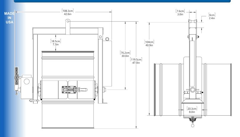
NOTE: Standard loop of pull chain extends approximately 6 feet (1.8 m) below the chain wheel
