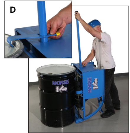
D. Extend tipping lever (1) fully and engage chine hook (2) on top rim of drum
