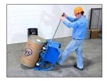
Simple Rock-Over Loading Built-in tipping lever facilitates loading. The tipping lever will only engage a drum that is 30" (76.2 cm) or taller.
