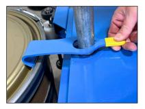
**Top Rim Hook** Engage Hook on top rim of drum to help in tipping it over into rolling position
