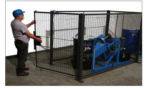
4. Close enclosure gate. Integrated safety interlock prevents drum rotation until the gate is closed, and automatically stops drum rotation if gate is opened during operation.
