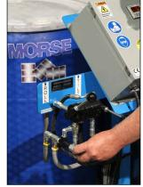
9. Adjust drum rotation from 4 to 16 RPM
