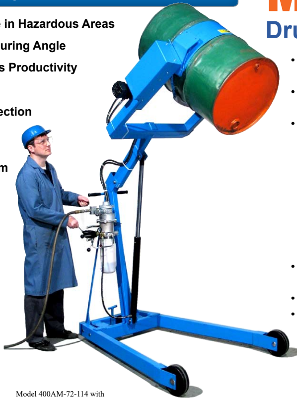
Model 400AM-72-114 with 72" (183 cm) dispensing height and AIR power lift and tilt.
