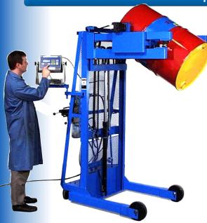
Model 515-T-114 shown is equipped with an intrinsically safe scale and air powered lift and tilt.
