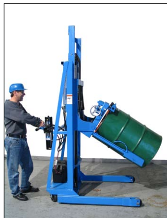
3. Tilt your drum to horizontal, then transport it to the desired location.
