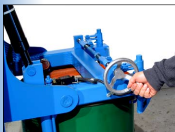
1. Secure the clamp to grip your drum.
