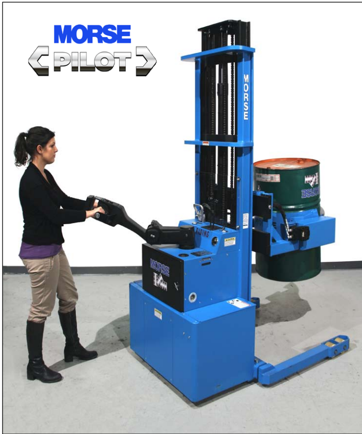
MORCINCH Drum Holder shown with standard Cinch Chain and Ratchet has flexible chain cover
