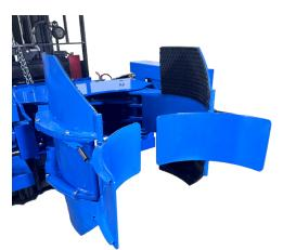
Larger Grip Pads to handle a plastic or fiber drum provide 75% more grip surface and allow higher grip pressure. Grip surface is high friction SBR Rubber Polymer (also known as RMA Grade II rubber).
