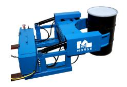
Grab a drum off pallet, floor, rack, etc. Grip drum with 8" x 16" (20 x 41 cm) jaws. Heavy duty hydraulic grip cylinders include a velocity fuse to provide a full line shut-off in the event of a line failure.
