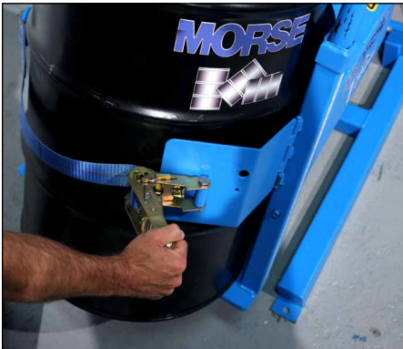
Secure drum in holder using web strap and ratchet around drum and tightening the two top clamps
