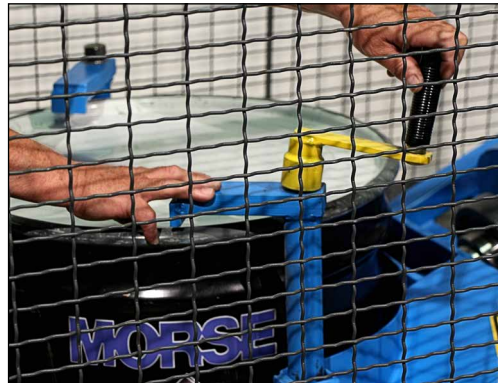
Secure drum in holder using web strap and ratchet around drum and tightening the two top clamps
