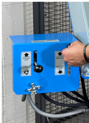
Use TILT handle to raise the drum into rotating position
