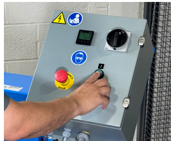
Push START button to activate power
