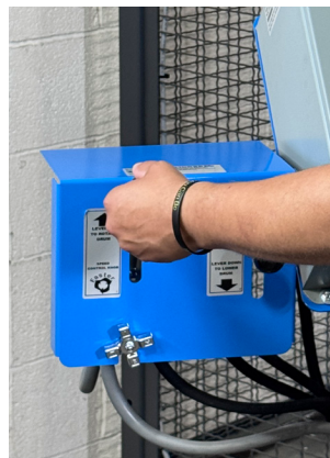
Use the ROLL handle to begin drum rotation
