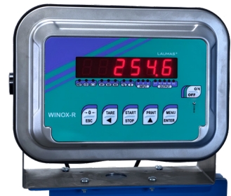
"T" Type Intrinsically safe scale indicator for use in hazardous areas.
