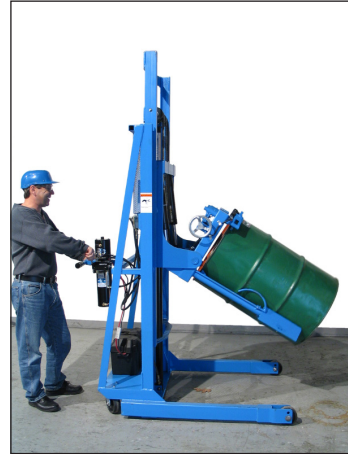
3. Tilt drum to horizontal. Transport racking location.
