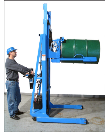
4. Release clamp from horizontal drum. Then raise drum to place on rack up to 8.5' (2.59 m) high.
