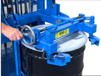
1. Manually secure clamp to grip drum under top rim.
