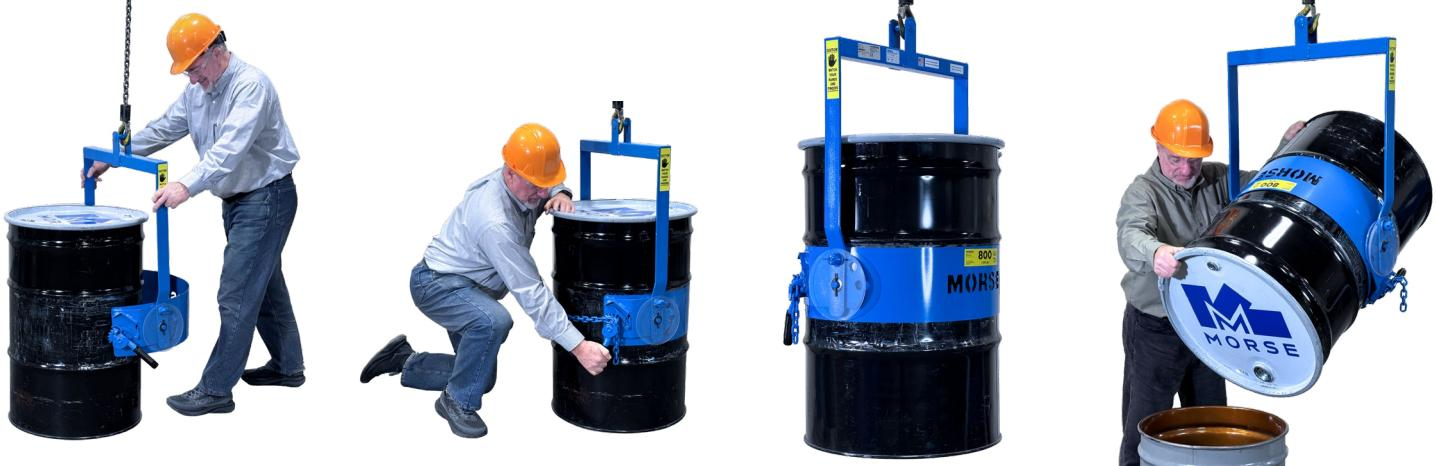
Suspended Drum-Karrier from hook. Push so drum holder engages between drum ribs.
