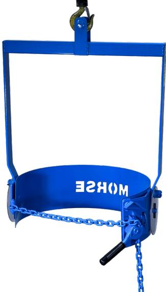
Built with welded structural steel for long service. Use tilt locks at each side of frame to lock drum in upright position. Can also lock in horizontal or 45° position to pour. When unlocked, manually tilt drum by hand tilt to any angle to dispense contents. Rotate drum by hand 360° in either direction.
