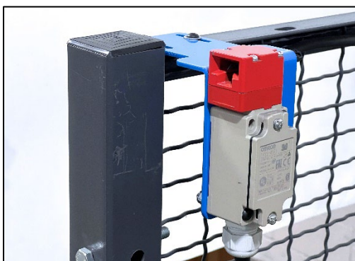
Mark where to drill holes in top of side panel for switch mounting plate.
