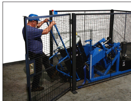
Load with drum truck at floor level
