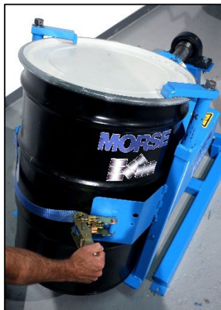
Tighten web strap around drum
