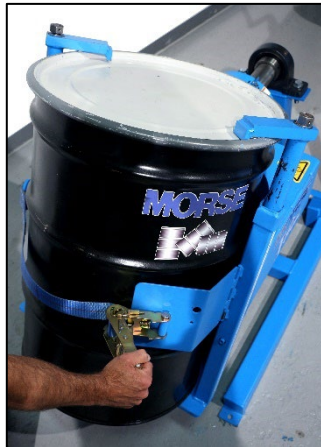
Tighten web strap around drum
