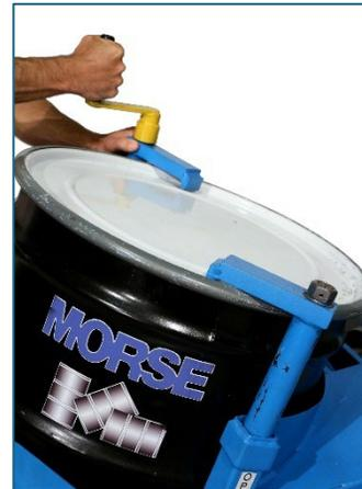
4. Turn the top clamps until they tighten against top of drum. Then remove hand crank BEFORE rotating drum.
