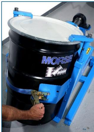
3. Drape the web strap across the face of the drum, and thread through slot in ratchet. Operate ratchet to tighten strap around drum.
