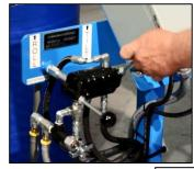
Place an upright drum onto the load plate with a drum truck or with your crane and a below-hook drum lifter.
