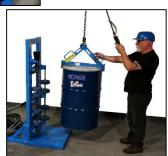
2. Lower the "TILT" lever to tilt the drum from upright into horizontal position.
