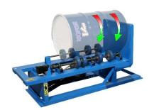
5. The drum rotation speed can be varied with the metering valve (item 13 on page 9). Turn the valve clockwise to increase speed up to 16 RPM, counter-clockwise to decrease speed down to 4 RPM.
