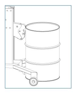
3. With drum held off the floor, push drum lifter to deliver drum. Avoid unreasonably rough or non-level surfaces. Move at moderate speed. Carry drum only high enough to avoid contact with the floor or obstacles. Push (rather than pull) loaded unit when possible for transporting. Pulling unit should be limited to maneuvering at short distance.
