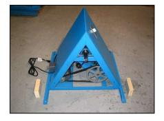
Step 5: Place a  $2 \times 4$  (51  $\times 102$  mm) spacer on each side of the frame, these will be used to hold the back panel of enclosure 3.5" (89mm) off the floor.
