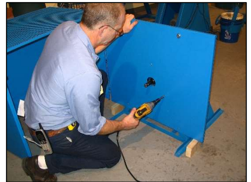
Step 9: Adjust the three casters so bottom of cage is approximately 4" (102mm) off the floor. Do not lock in place yet. Close enclosure and verify that the key aligns properly with the switch. If key is not aligned properly adjust casters accordingly. Key may also be adjusted by loosening its screws and moving. Once key is aligned properly, lock casters in place by tightening jam nut upward.
