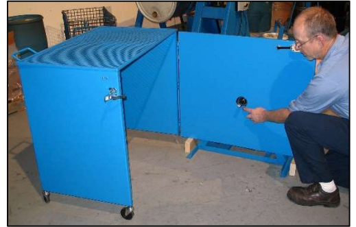
Step 7: Align each self drilling screw near the center of the angle frame.
