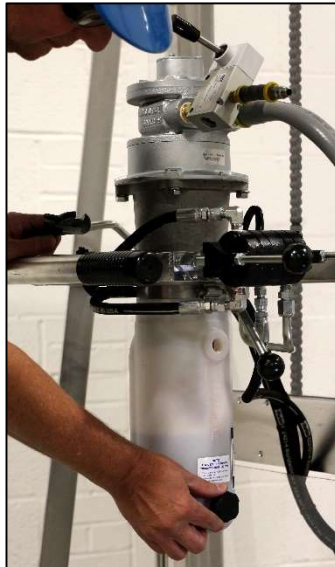
Remove BLACK breather from storage position
