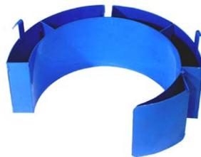
Diameter Adaptors for drums from 18.5" to 22" in diameter do not have hold-down brackets. They fit between the ribs of a steel drum. For plastic or fiber drum, use Diameter Adaptor in combination with the Bracket Assembly to prevent the drum from slipping lengthways through the drum holder.
