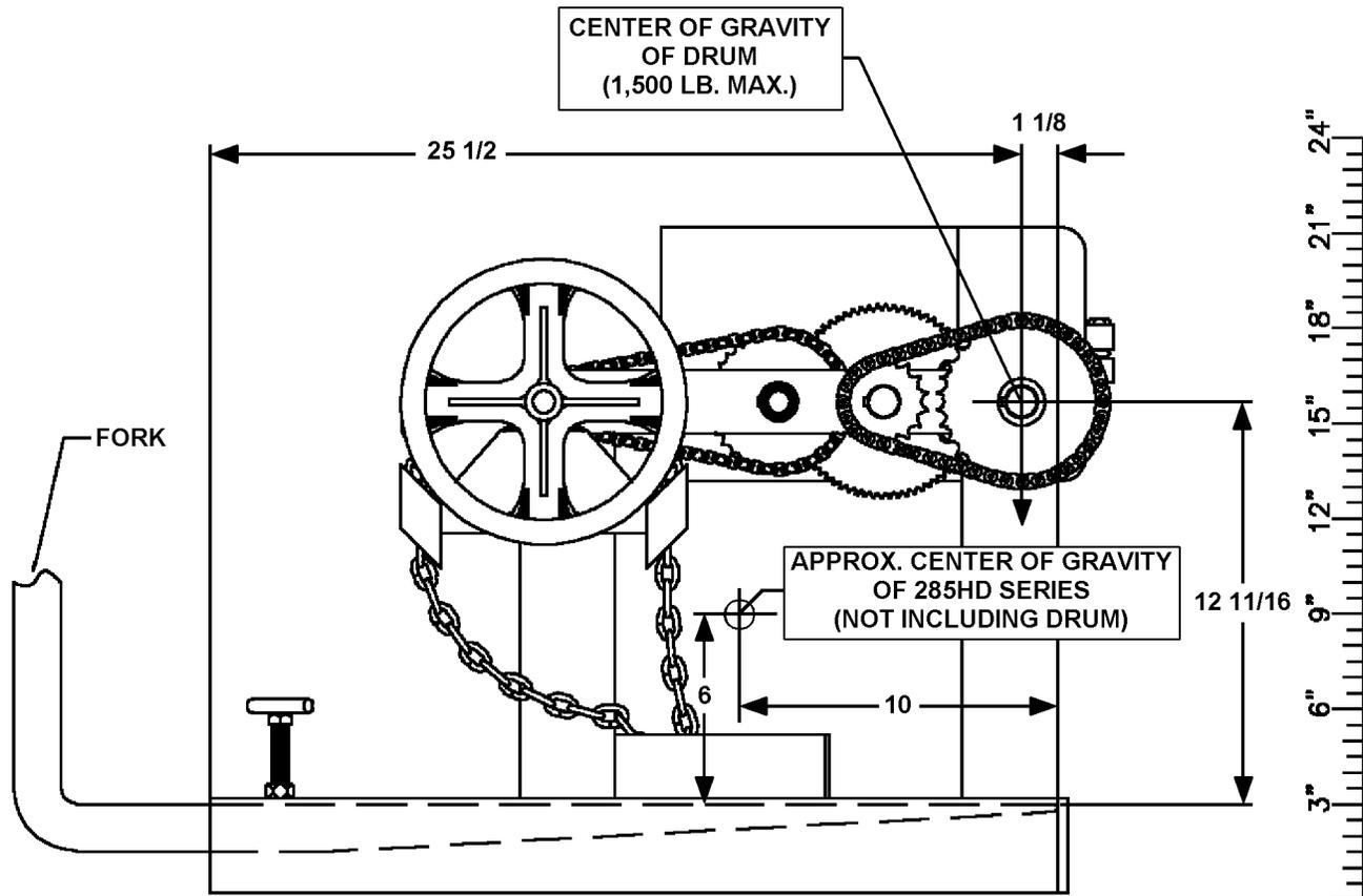
DIMENSIONS ARE MEASURED FROM INSIDE OF FORK TUBE END. THIS WILL GIVE A FIXED POINT TO WHICH LOST LOAD DATA CAN BE DETERMINED. (FORKS MUST BE TOUCHING THIS FORK TUBE END.)
