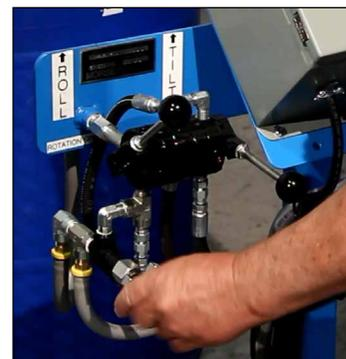
Alternate method on the air motor version: With the air shutoff ball valve in the OFF position, raise the ROTATE valve to the ROTATE position. Then, slowly open the air shutoff ball valve to begin the rotation. This can allow for more control over the speed of rotation.
