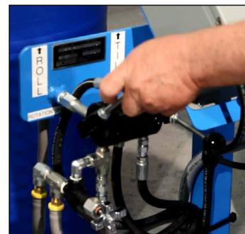
4. The drum rotation speed can be varied with the metering valve. Turn the valve clockwise to increase speed up to 20 RPM, counter-clockwise to decrease speed down to 5 RPM.
