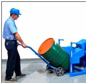
Load drum with drum truck
