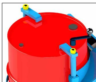
4. Turn the top clamps until they tighten against top of drum. Then remove hand crank BEFORE rotating drum.
