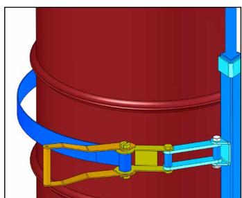
3. Drape the web strap across the face of the drum, and thread through slot in ratchet. Operate ratchet to tighten strap around drum.
