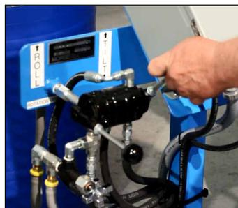
2. Raise the drum to the top position by raising the "LIFT" lever, on the right.
