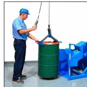
Load drum with hoist attachment
