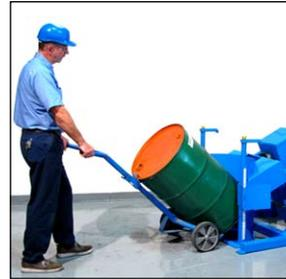
Load drum with drum truck
