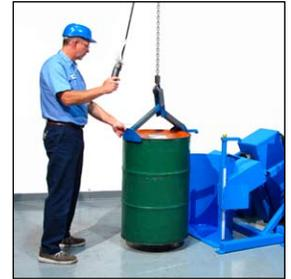
Load drum with hoist attachment
