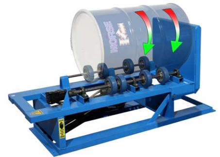
5. The drum rotation speed can be varied with the metering valve (item 13 on page 8). Turn the valve clockwise to increase speed up to 20 RPM, counter-clockwise to decrease speed down to 5 RPM.
