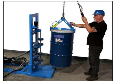
3. Lower the "TILT" lever to tilt the drum from upright into horizontal position.
