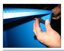
Step 9: Adjust the three casters so bottom of cage is approximately 4" off the floor (shown right). Do not lock in place just yet. Close enclosure and verify that the key aligns properly with the switch. If key is not aligned properly adjust casters accordingly. Key may also be adjusted by loosening its screws and moving (shown left). Once key is aligned properly, lock casters in place by tightening jam nut upward.
