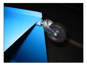
Step 4: Install casters to enclosure if necessary.
