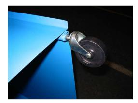
Step 4: Install casters to enclosure if necessary.
