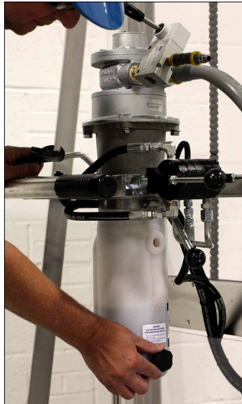
Remove BLACK breather from storage position
