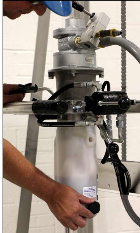
Remove BLACK breather from storage position
