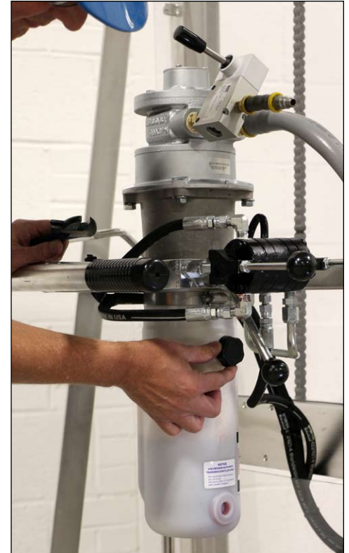
Install BLACK breather in place of RED shipping plug
