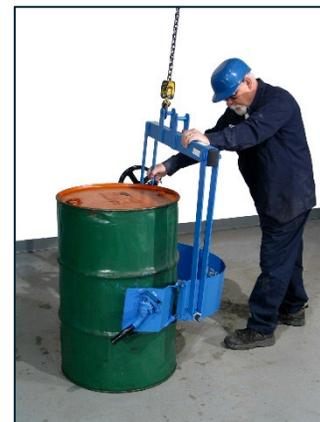
6. Move hoist hook to lift point centered over drum.
