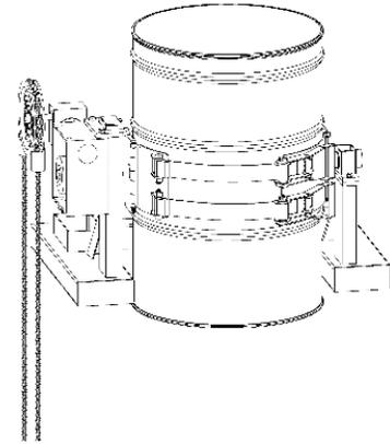
7. Raise forks to clear floor and transport drum in vertical position to dispensing location.
